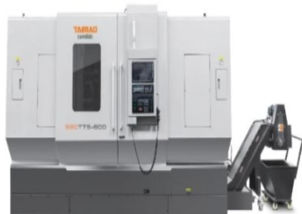
**High rigidity and stability**-- by adopting the flat bed, 30-degree inclined guide rail, and reinforced rib design, the distortion and thermal deformation can be minimized.
