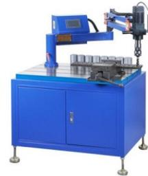
Another infrequent product present in YME 2024 was the high-speed CNC drilling & milling machine, which was mainly used for the drilling, milling, tapping, reaming and boring of the structural parts such as flanges, flat plates and automotive components. The entire process was digitalized, with easy operation and high efficiency.
