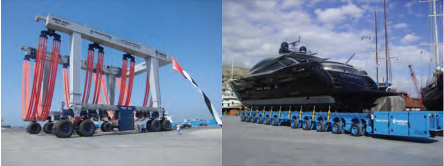
Cimolai Technology Spa supplies customized mobile boat hoists ranging from 30 t to 2000 t diesel and full electric, ship lifting platforms "cimolift" to launch and dry-dock huge vessels, special cranes to move, lift and turn ship blocks, self-propelled modular trailers spmt and transfer systems to support the "cimolift" or to be used independently to perform the transportation and parking operations of the vessels within the shipyards.
