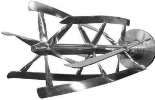
Since 1964 ZUCCHETTI designs and manufactures a wide range of customized industrial agitators and mixers for critical applications accordingly to the specifications of worldwide recognized licensors of ABS/HDPE/LDPE/PE/PET/PP/PTFE/PVC/SBR.
